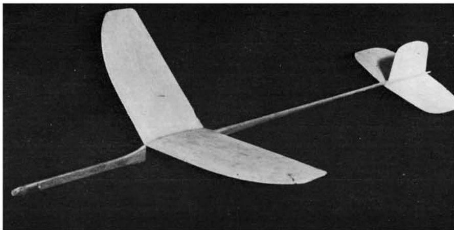
For a minimum of expense Rain Crow returns a maximum of exhilarating flying fun. The wing does have different amounts of twist on each panel at various stations—and a bit of rudder offset. Slim fuselage is cut and shaped from spruce, so it's tough enough for any scramble.
